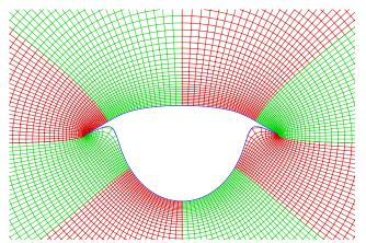
Fig. 10 Computational grid for the cobralike forebody in the exit plane.
