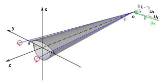
Fig. 1 Slender conical wing-body combination and separation vortices.
